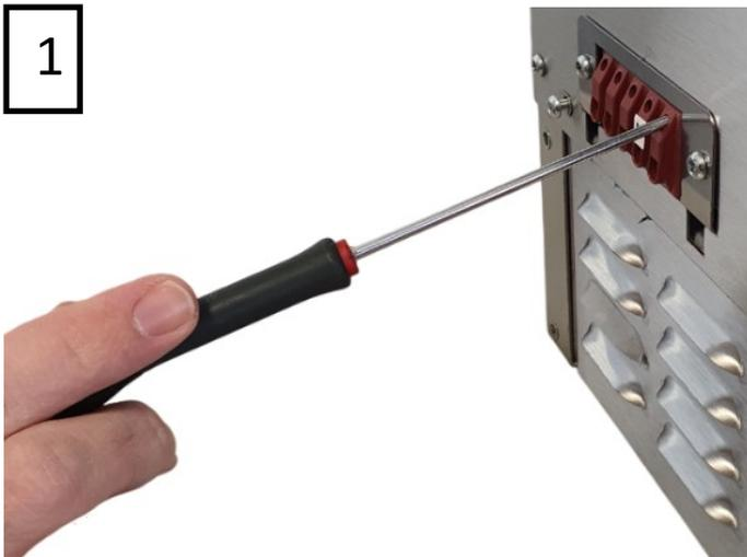
2 - Then lift the screwdriver to open the terminal block's spring-loaded jaw and insert your conductor into the terminal block's lower housing:
